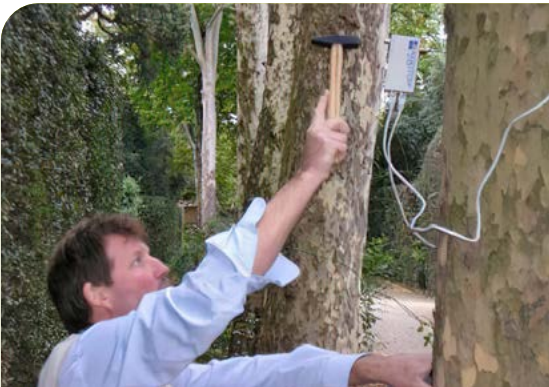
Execution of survey for the verification of the tree stability with tomography instrumentation. © Saverio Lastrucci.
